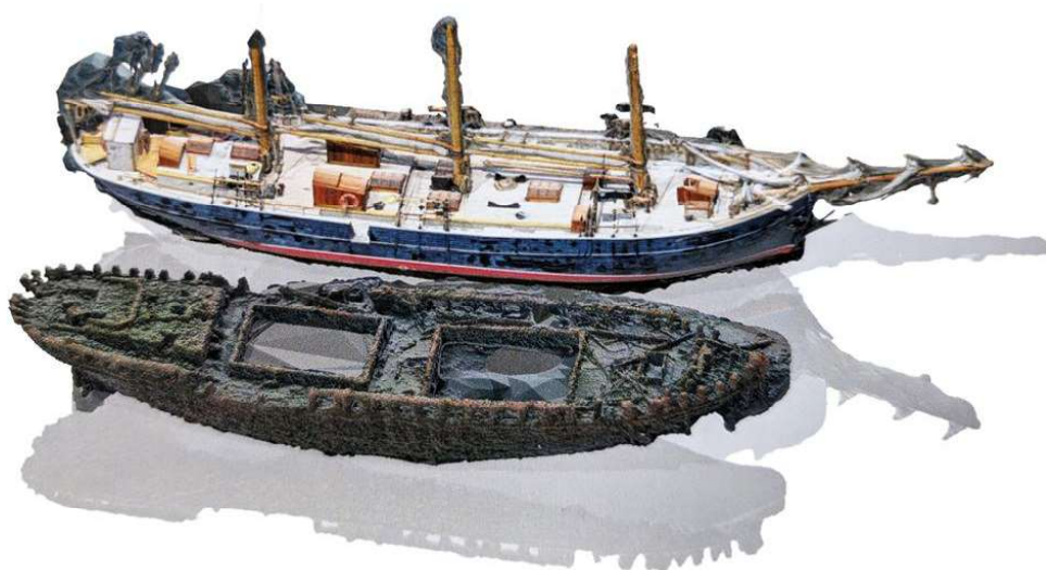
Figure 2: Comparison between the photogrammetry models of the still existing sister ship and the “Lehnskov”.
